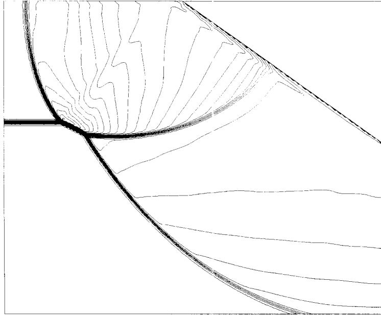
Figure 6. (e) Holographic interferogram of the wave configuration at a longer time after the head-on collision of the regular reflection with the end-wall. M_1 = 1.263 , \theta_w = 55^\circ . (f) Numerical simulation of the wave configuration shown in Figure 6(e). M_1 = 1.263 , \theta_w = 55^\circ .
