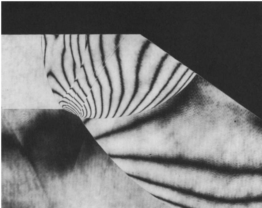
Figure 6. (e) Holographic interferogram of the wave configuration at a longer time after the head-on collision of the regular reflection with the end-wall. M_1 = 1.263 , \theta_w = 55^\circ . (f) Numerical simulation of the wave configuration shown in Figure 6(e). M_1 = 1.263 , \theta_w = 55^\circ .
